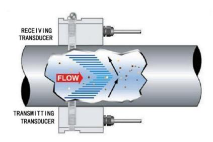
The presence of large enough particles in the liquid is necessary to generate a longitudinal reflection. The particle size must be greater than 100 microns.
